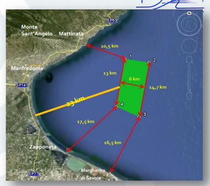
The project GARGANO SUD, is based on 85 wind turbines of 4 MW each, for a total of 340 MW installed.
