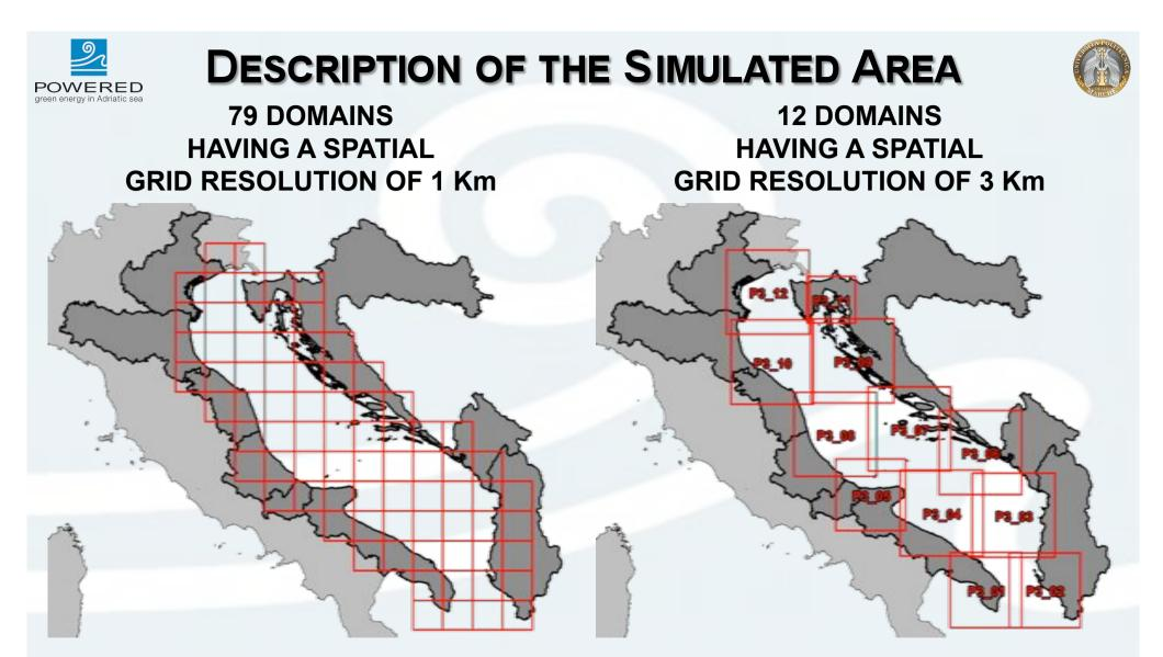
Long term analyses are actually obtained with a 3 [km] resolution for the years from 2008 to 2011, while 1 [km] simulations are carried out for the 2010 year.
