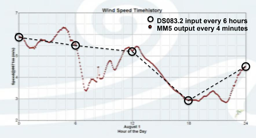
Using the MM5 code is possible to describe the wind behaviour in the period separating two DS083.2 input. This is very useful especially to evaluate the wind turbine energy production.
