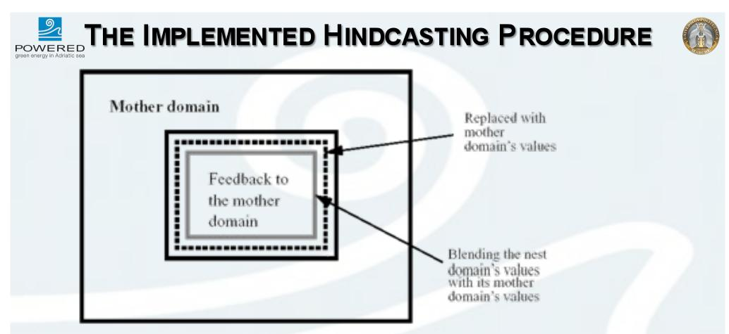
The hindcasting analysis is implemented with a **two way nesting** procedure. In this way the initializing meteo data are ingested by the coarser mother domain and they propagate to the finer nested domains; at the same time the more accurate results of the nested domains are fed back to the mother ones so to improve the global solution accuracy.
