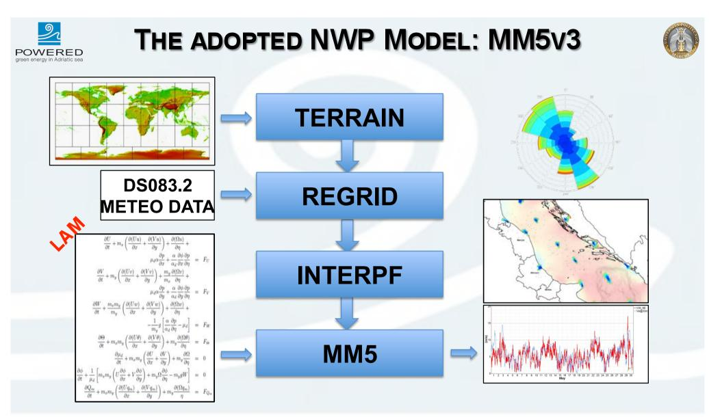
"The PSU/NCAR mesoscale model (known as MM5) is a limited-area, nonhydrostatic, terrainfollowing sigma-coordinate model designed to simulate or predict mesoscale atmospheric circulation."
